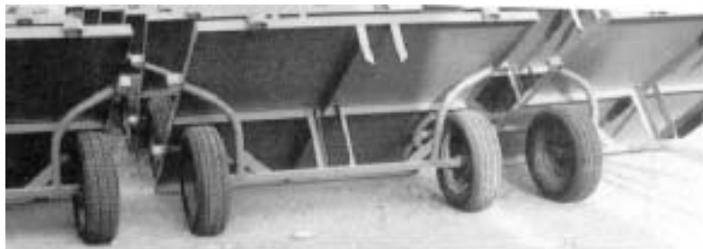
Figure 28: Two-wheel carts using roller bearings and factory-reject car tires. Designed for a team of oxen, but a smaller size is used with donkeys in Togo.
